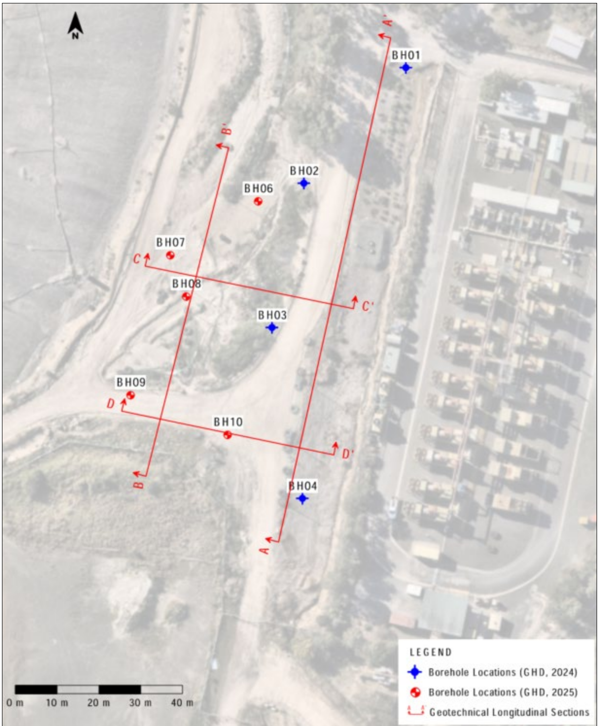
Figure 4.5 Locations of geotechnical investigation boreholes (GHD, 2024)
