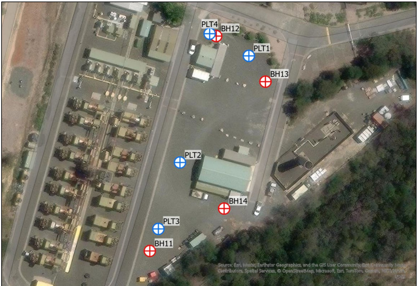
Figure 4.4 Location of geotechnical investigation boreholes (GHD, 2025)
